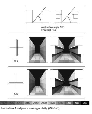
Figure 5: Incident Solar radiation received on street of different geometries. [5]
