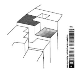
Figure 10: Insolation Analysis on a terrace of the detailed block illustrating the reduced incident solar radiation due to overshadowing by adjacent terraces. [5]
