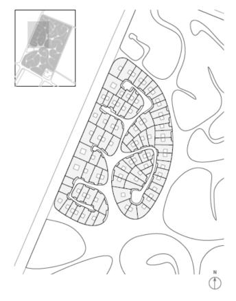
Figure 9: Detailed Plan of a section of the proposal showing the plot divisions, plot entrances and courtyards
